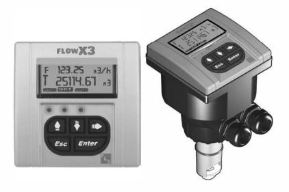
FLS FLOWX3 F9.00 Flow Monitors & Transmitters are designed to convert the signal from all FLOWX3 flow sensors into a display indication and a 4-20 mA signal for long distance transmission. A very simple and complete choice of options are granted by single or dual input/output, two solid state relays output and one relay output.
