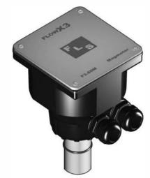
The FLOWX3 F3.60M & F3.63M Insertion Magmeters are suitable to measure flowrate in both metal and thermoplastic pipelines. No moving mechanical parts and the high quality materials allow the measurement of liquids where suspended solids can be present or of abrasive liquids as long as they are conductive and homogeneous.
