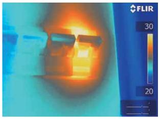
Thermal image of an overheated fuse.
