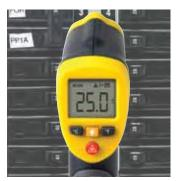
IR thermometer, temperature measurement FLIR i3, temperature in 3,600 spots
