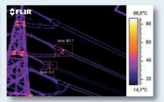
Image taken with 320  $\times$  240 pixels resolution and 50mK thermal sensitivity. Please note how the increased number of pixels will result in a more accurate temperature reading in the hot spot.
