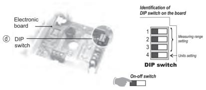
To configure the transmitter, it must not be energized. Then, you can make the settings required, with the DIP switches (as shown on the drawing beside). When the transmitter is configured, you can power it up.
