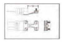
Stainless steel wire clamp bracket for miniature or standard connectors
