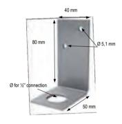
**BF-M**: Stainless steel (316 L) wall fixing support. Delivered with a  $\frac{1}{2}$ " G screw nut.
