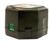
KI - AL - 100 C : Class 2 power supply for sensors, Input voltage : 230 Vac, Output voltage : 24Vdc, intensity 250mA.
