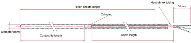
Teflon sheath length = Contact tip length + cable length
