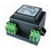
KI - AL - 100 A: Class 2 power supply for **\$G100** sensors. Mounting with integrated brackets. Input voltage: 230 Vac, output voltage 24Vac, intensity 100mA.
