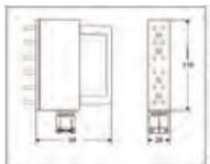
Multiple connector for thermocouple. Suitable for the simultaneous connection of 1 to 6 standard circuits.
