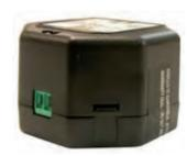
KI - AL - 100 C: Class 2 power supply for **SG100** sensors, Input voltage: 230 Vac, Output voltage: 24Vdc, intensity 250mA.
