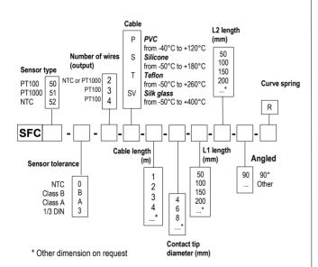
Example: SFC-51-B-2-P-1-4-100-100-90-R Model: PT1000 temperature probe class B, 2 wires, PVC cable of 1m length. Stainless steel contact tip Ø 4 mm angled at 90° and L1 and L2 lengths of 100 mm, with curve spring. Measuring range from -40 to +120°C.
