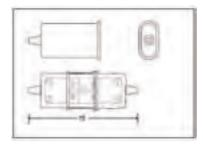
For wet use, good vibration resistance. **Temperature resistance**: 200 °C
