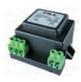
KI - AL – 100 A: Class 2 power supply for sensors. Mounting with integrated brackets. Input voltage: 230 Vac, output voltage 24Vac, intensity 100mA.
