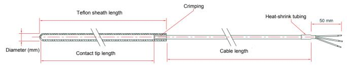
Teflon sheath length = Contact tip length
