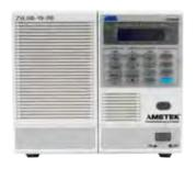
Traditional dc Electronic Load Solutions have inherent limitations for testing single cell fuel cells and PV cells/modules. DC electronic loads use power dissipating components that require a minimum compliance voltage of 0.6Vdc  $\sim$  1.5Vdc for operation. However, single cell fuel cells and PV cells often require the dc electronic load to operate at below 0.1Vdc. The ZVL was designed to address all of these needs.
