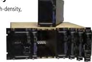
provide programmable stimulus, bias power, and loading for devices under test (DUTs).
